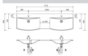
Washing stands without anchoring brackets have to be fixed on the wall and on the furniture-side with silicon!
