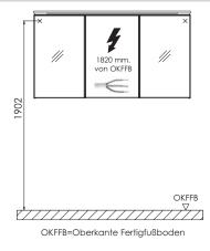
For washing stands with fixing screws, the dimensions for boring must be drawn in on-site after the washing stand has been laid on the floor unit.
